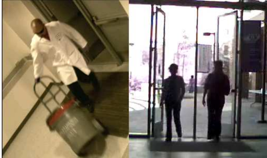
Figure 6.5: The left panel shows an example of a double count at the loading dock entrance of the building; the right panel shows an example of a missed count at the front door.
