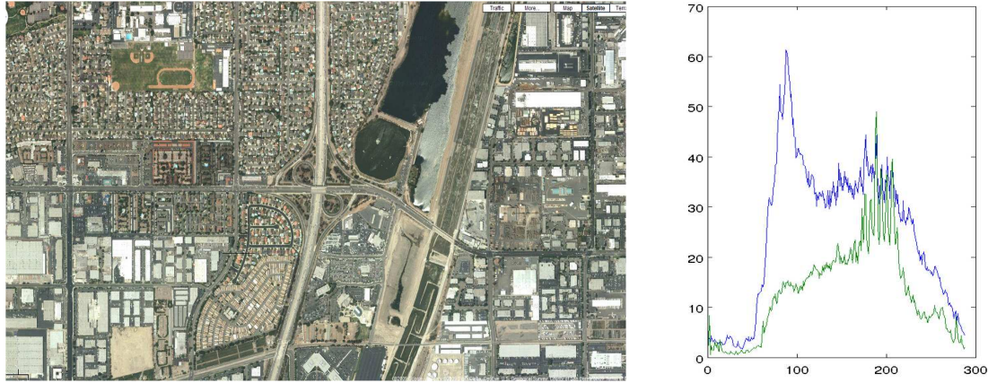
Figure 8.13: The interchange in the middle of the satellite image on the left has two on-ramps for entering the North Freeway. The flow profile for the on-ramp that is fed by traffic approaching from the largely industrial region to the east of the ramp is in green in the plot on the right; and the flow profile for the on-ramp that is fed by traffic approaching from the largely residential region to the west of the ramp is in blue.
